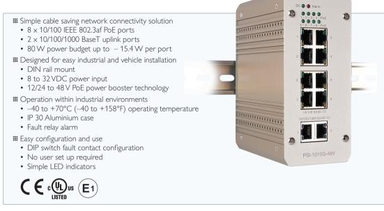
PoE technology is designed to eliminate the need for separate installation of power cables to equipment. Power is provided to equipment over the UTP data cabling. The PSI -1010G-24V is a simple PoE switch capable of driving 8 connected devices as well as two Gbit uplink ports for the most bandwidth intensive applications.
